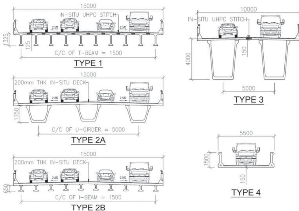
**Fig. 1.** Four different types of Dura® UHPC bridge girders.
