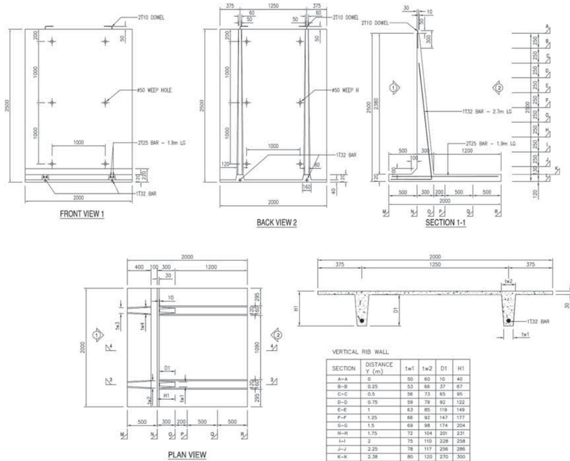
Fig. 9. Detail of UHPC retaining wall.
