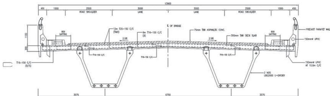
Fig. 5. Typical cross-section of KB-KT Bridge.
