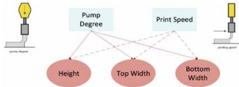
**Fig. 5.** Simple scheme of printer parameter and geometry parameter relations.
