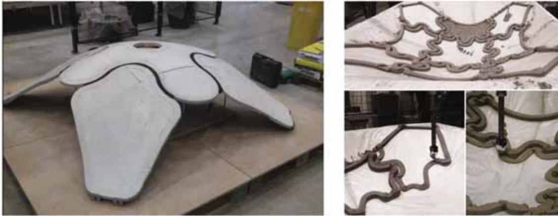
**Fig. 12.** Printed compression shell (3TU Lighthouse 2016 project, TU/e with TU Delft).
