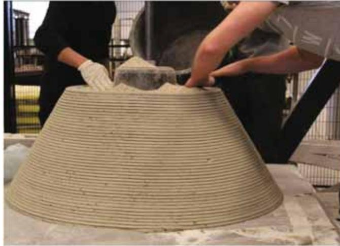
**Fig. 11** Example of a simple type of vault printed with an unbounded Material (coarse sand).
