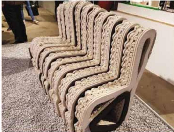
**Fig. 19.** Prestressed printed concrete street furniture
