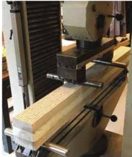
**Fig. 16.** Printed sandwich beam in 4-point bending.
