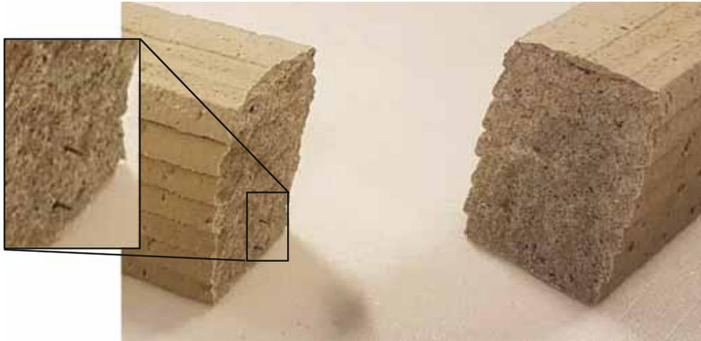
**Fig. 15.** Printed beam after testing.
