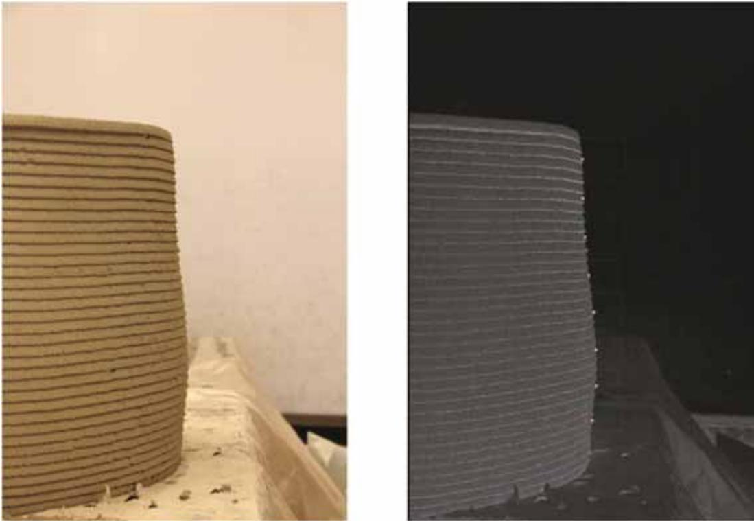
**Fig. 9.** (a, b) Tracking deformations of a printed object with optical measurements.
