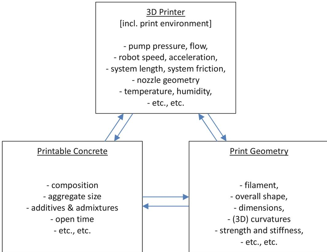
**Fig. 3.** Interdependency of system parameters (selection) of the 3DCP system.
