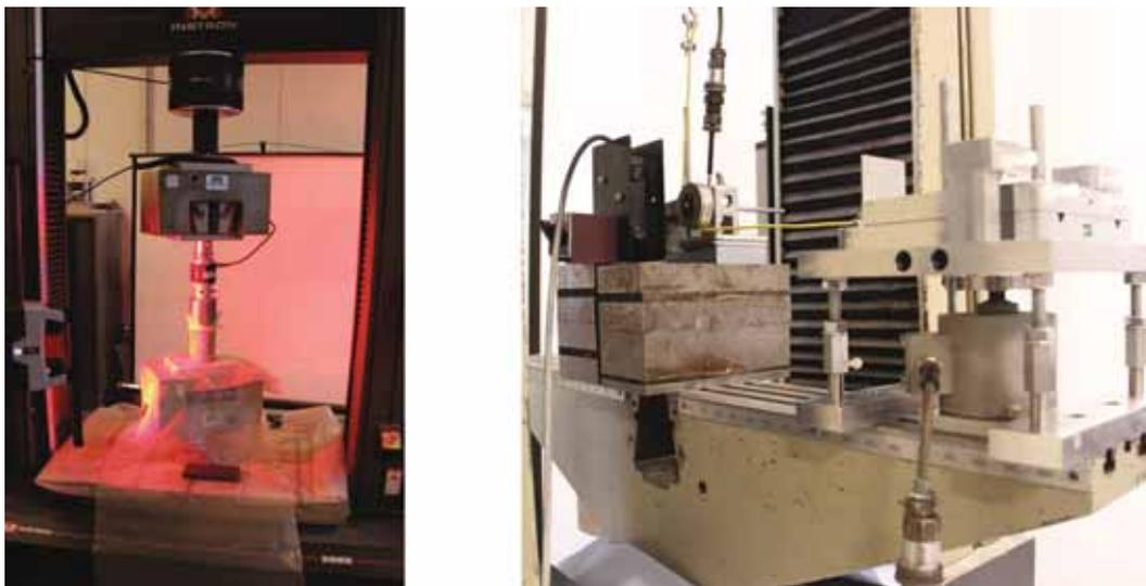
**Fig. 8.** (a, b) Custom developed uni-axial compression test and shear box test.
