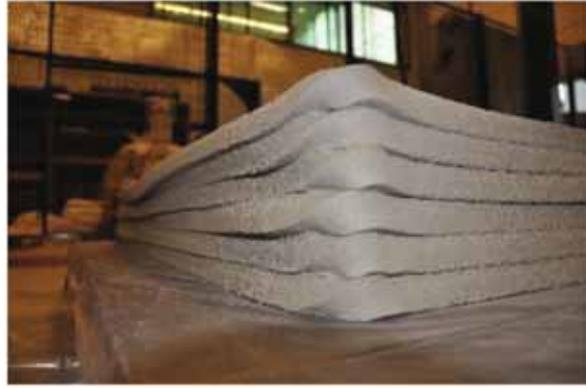
**Fig. 2.** Twisting of the filament occurs when a non-circular nozzle does not stay aligned to the print path direction.
