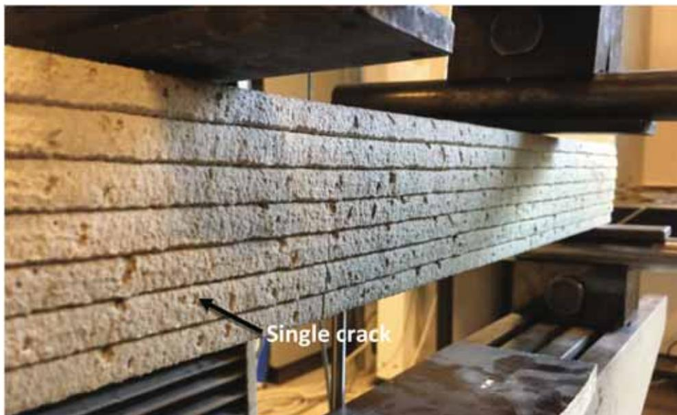
**Fig. 14.** Printed beam with embedded cable reinforcement in 4-point bending.
